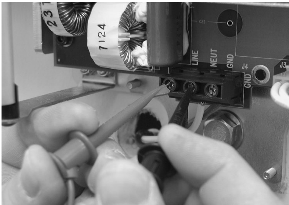
Figure 31 Verifying Input Voltage at the Line Input
