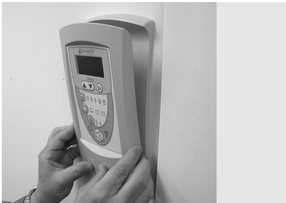
Figure 38 Snapping the Operator Panel to the Mounting Cradle
