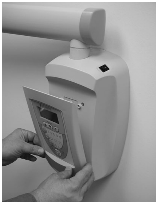
Figure 37 Snapping in the Operator Panel
