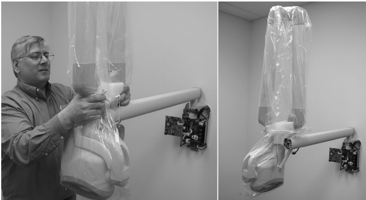
Figure 20 Installing the Articulating Arm and Tubehead Assembly
